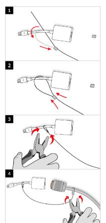
Starting with a single cable tether and two (2) metal sleeves, insert the TetherTies® wire through one end of one metal sleeve. Loop wire around the item vou'd like to secure. Feed wire down the other hole of same metal sleeve until it is even with the bottom of sleeve.
