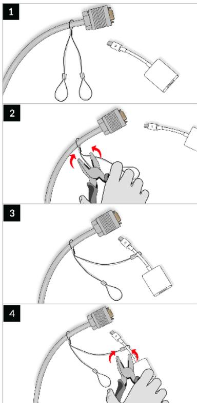
1 Slip a loop from one end of your TetherTies® Multi-Adapter over the end of the adapter, cable, or other item you'd like to secure.
